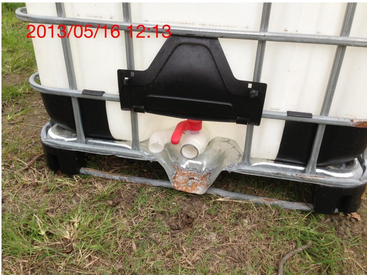
**Photo of the open IBC tap, and the spilled chemical on the ground where the reaction took place.**
