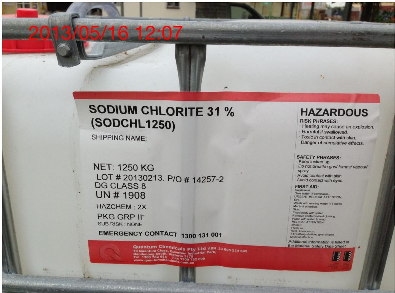
**Evidence photo of container label, the investigator is able to follow up with the confirmation of the contents from the SDS. (Safety Data Sheet)**
